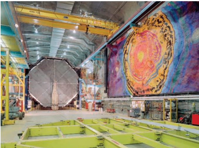
Bull's-eye. Steel plates in an underground lab in Minnesota are designed to capture neutrinos from Fermilab, 700 kilometers away.
